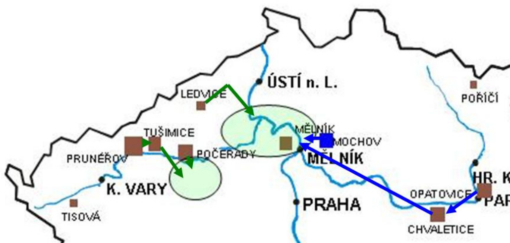
Figure 5.2 CO 2 transportation routes – scenario 1, 2030-2044; green: infrastructure built during 2025-2029
